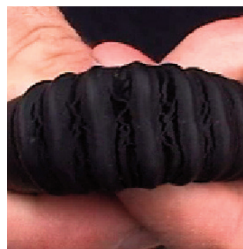
By bending hoses and short milk tubes you can see cracks and tears, especially where these items bend or are pinched by shut-offs.
